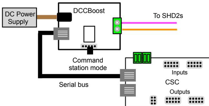
The DCCBoost can be used with the Team Digital Central Signal Controller (CSC). In this application the DCCBoost is set for command station mode. The DCCBoost receives signal message from the CSC and converts them into DCC packets to control Signal Head Decoder 2s (SHD2). In the command station mode the data and ground pins are used. Use a 6 wire cable that will plug into the DCCBoost and a CSC.
