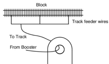
Locomotives and lighted cars draw enough current to trigger the DBD22. In order for other rolling stock to draw current, resistive wheel sets will have to be added. For HO scale (14 volts), one 4.7K ohm resistive wheel set will work per car. For N scale (12 volts), one 3.9K ohm resistive wheel set will work per car. If you want to use 10K resistive wheel sets you will need two or three wheel sets per car depending on track voltage. See specifications.
