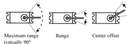
3. Program CV7 with a value of 2 to put the servo in the center position.
