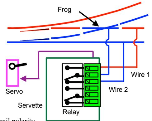
The relay wiring shown is very close to the actual except for Wire 1 and Wire 2. These wires may have to be reversed at the relay terminals so that the correct rail polarity gets to the frog. This will be determined by the way the servo is mounted and linked to the turnout. Either set of relay contacts can be used for frog power.
